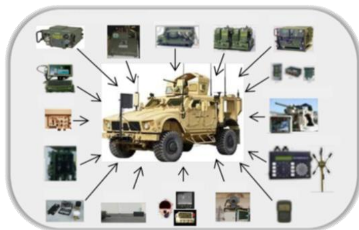
Figure 1. Legacy stovepiped systems consume an inordinate amount of SWaP on Army vehicles.
