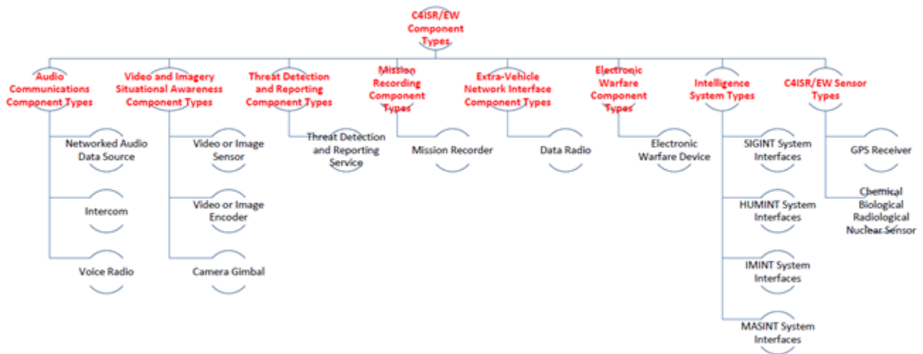
Figure 2. The VICTORY architecture defines component types for C4ISR/EW systems. Other component types include VDB component types and platform systems. Figure taken from the VICTORY Training Material [4].
